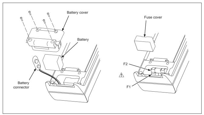
Figure 1. Battery and Fuse Replacement
